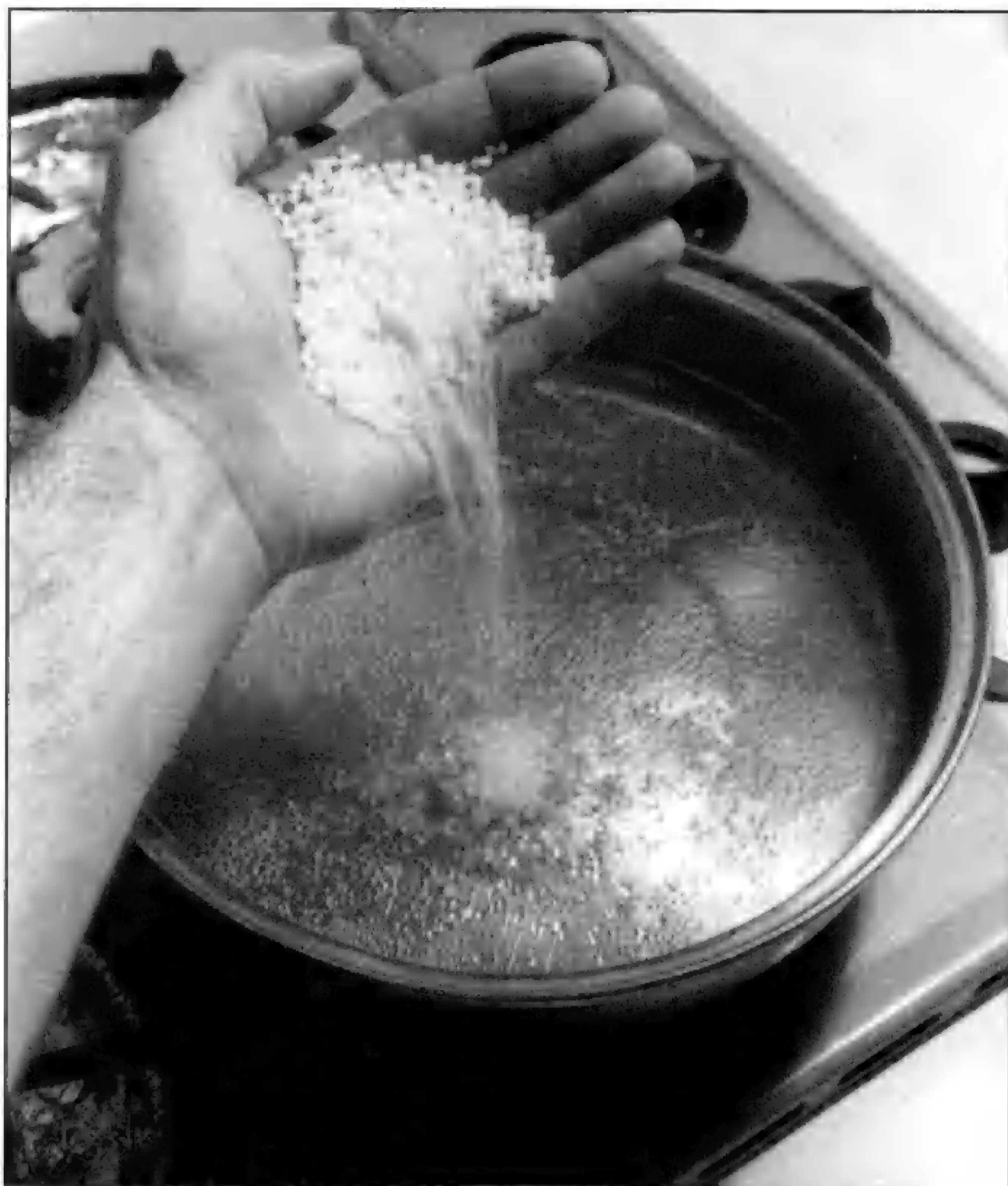
When Friendly Plastic is poured into hot water it turns into a clay-like, pliable material.
